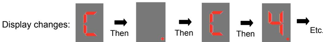
With Configuration C4 flashing in the display, along with the dot in the lower right corner, the Interface Adapter board is now configured to operate a **180/180 mm – 3.2kW** domino, which is the center configuration for our example (VICU266).
